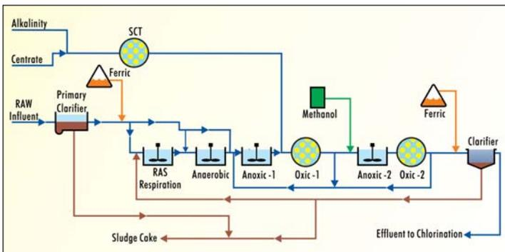
Typical BNR Wastewater Treatment Plant Setup in BioWin.
