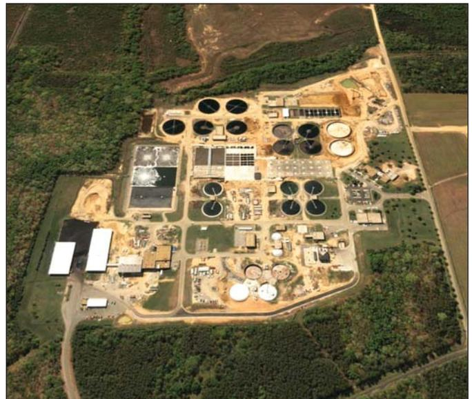
The Henrico County Water Reclamation Facility (shown above during construction and now completed) is a 75-mgd wastewater treatment plant located southeast of Richmond, VA. An initial upgrade, designed by Hazen and Sawyer, increased capacity, simplified the treatment process, and added BNR. We are now working with Henrico County to further reduce nutrients as part of the Chesapeake Bay ENR program.
