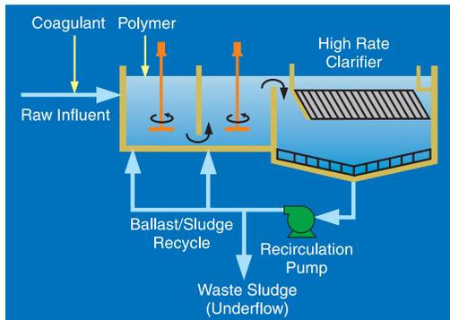
*HRPCT treats CSO at overflow rates at least 50 times greater than those of conventional settling tanks, while providing much better BOD and TSS removal.*
