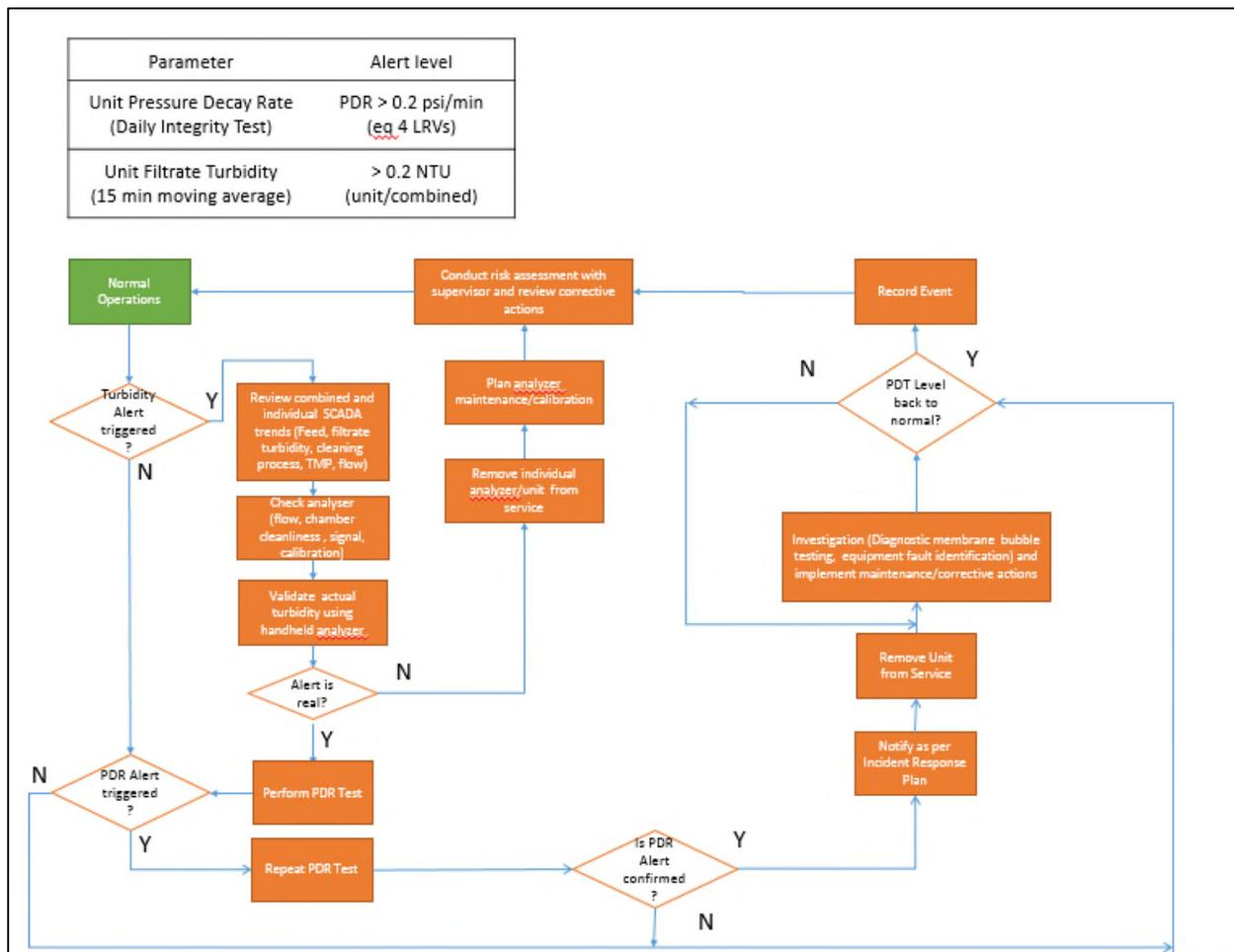
**Figure 1 - MF/UF Critical Response Procedure**
